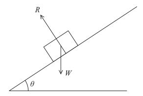
The diagram shows the forces acting on an object on an inclined surface.
