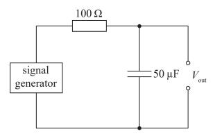
The graph shows the square wave output of the signal generator. The frequency of the square wave is 20 Hz.
