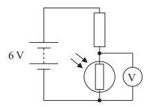
In daylight the voltmeter reads 3.0 V.
