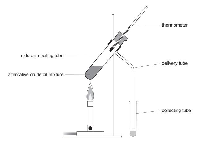
In her experiment, Lois gently heated  $10\,\mathrm{cm}^3$  of an alternative crude oil mixture in a side-arm boiling tube.
