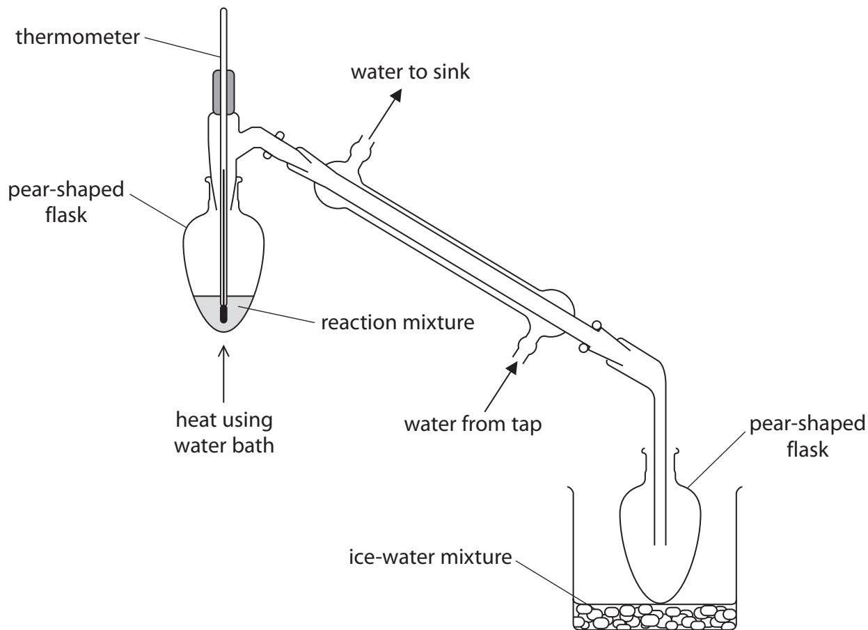
Discuss the improvements that should be made to the set-up of the apparatus. Include the likely effect of the errors identified on the yield or purity of the product.
